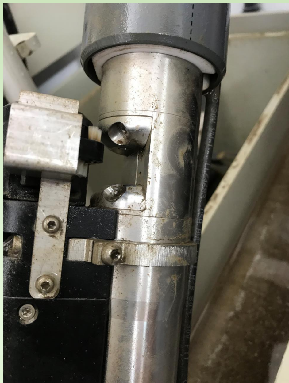
Figure 2: Online in-situ UV/Vis spectrophotometer equipped with automatic cleaning brush.
