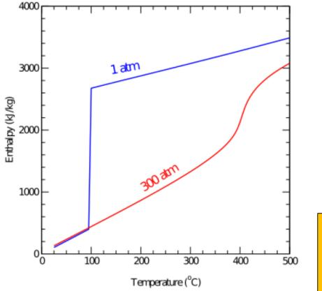
Available thermal energy expressed by the change in enthalpy ( $\Delta$ H) that can potentially be recovered by cooling water from reaction to room temperature.
