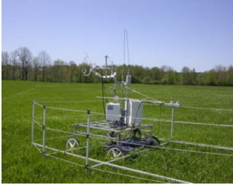
Eddy-covariance towers to measure ecosystem carbon balance
