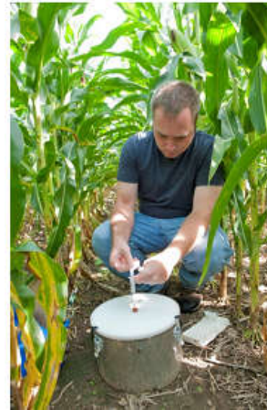
Static chambers to measure soil N_2O and CH_4 (GHG) emissions
