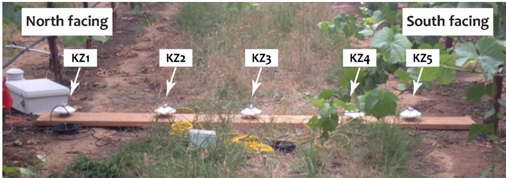
Relative locations of Kipp & Zonen radiation sensors
