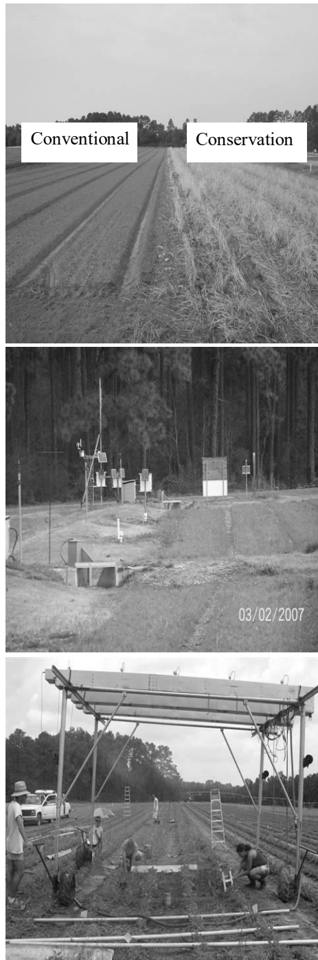
Figure 2: Plot scale experiments examine the effects of conventional versus conservation tillage on surface runoff and rainfall infiltration using whole plot flume and tile drain systems as well as rainfall simulation.
