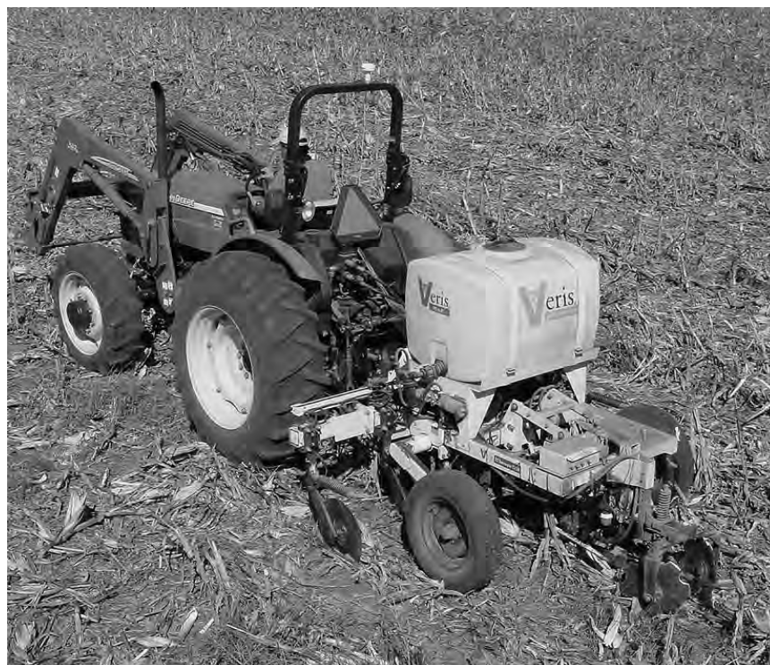
Fig. 3. Commercial sensor system integrating soil electrical conductivity and pH mapping (Veris pH manager, Veris Technologies, Salina, Kansas, USA).
